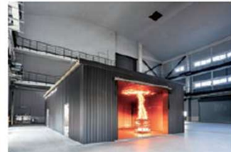
● Simulated Apartment Reproduction and verification of actual firefighting environments
