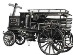
Developed Japan's first fire pump with a gasoline engine
