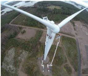
(windmill rotating shaft) of wind power generation facilities in North America is as high as 90 m, making the 104 m S341HLA an ideal solution.
